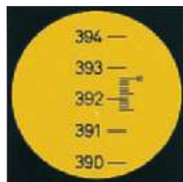
NAK2 circle reading (400 gon) 392.66 gon
